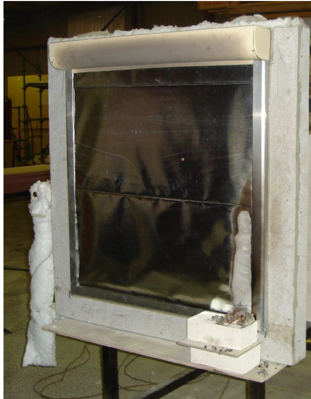
Figure A5.2: Specimen F after exposure to radiant heat and placement of crib.
