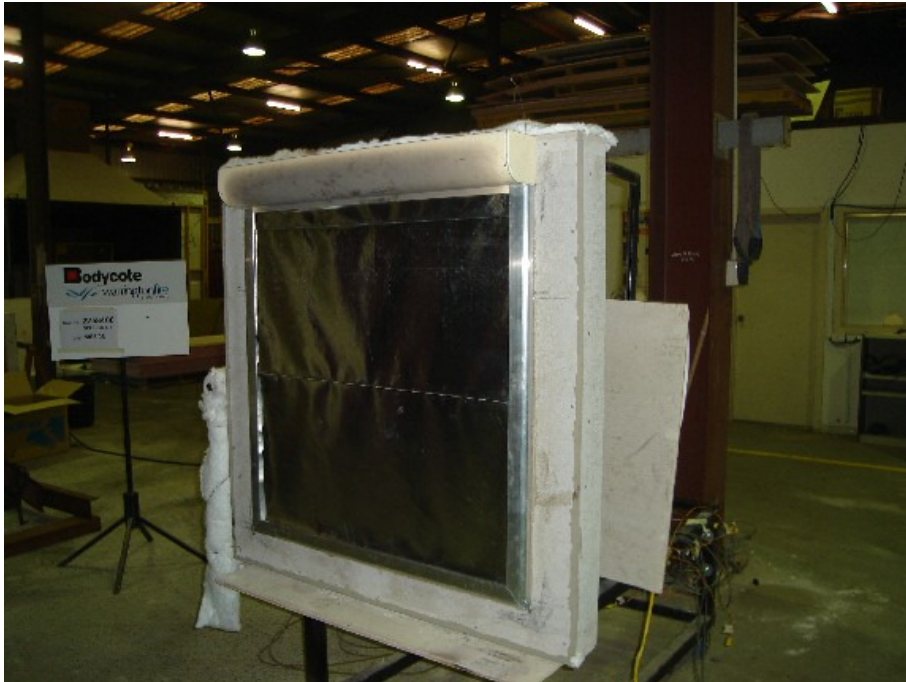
Figure A5.4: Specimen R after exposure to radiant heat.
