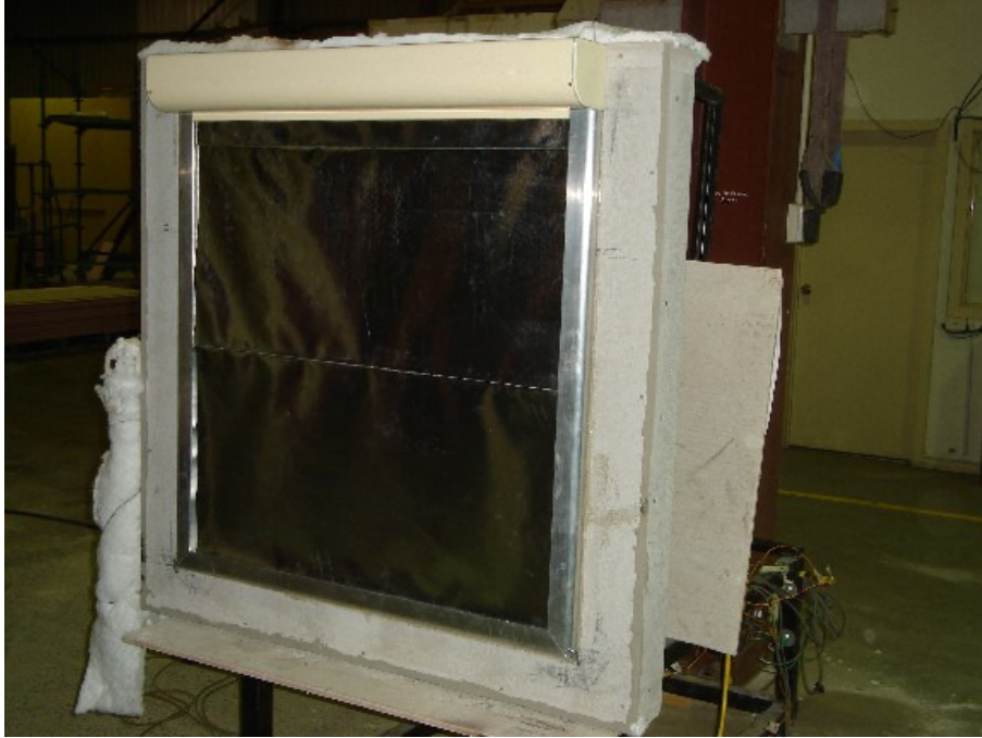
Figure A5.3: Specimen R before commencement of exposure to radiant heat.
