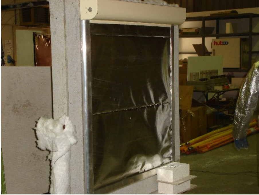
Figure A5.1 Specimen F before commencement of exposure to radiant heat.
